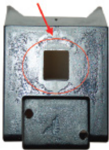
Rough Surface Finish
